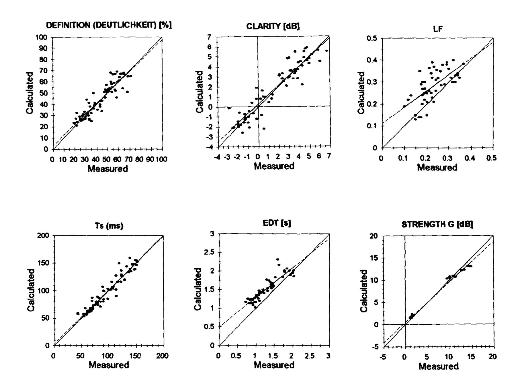
Fig. 1. Scatter diagrams of the room acoustical parameters. The unbroken line represents perfect agreement. The dashed line indicates the least squares fit to the data points (linear regression).
